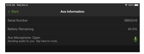
The Ava Microphone option reports the current status of the microphone in the Ava Robot. This is the microphone that picks up audio from the local environment which is transmitted to you, whether the video call is integrated into the app, or split to another app or endpoint. You can tap this entry to change the status.
