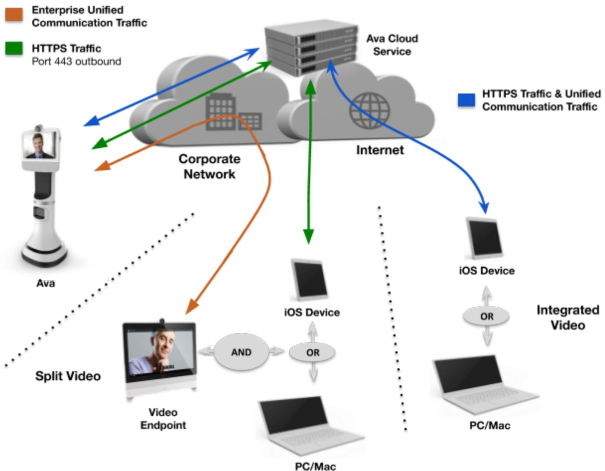
**Robot Operational Communications:** The Ava Control Application (Ava App) transmits operational commands from the remote user to the Ava Cloud Service, which in turn communicates with the Ava robot.
